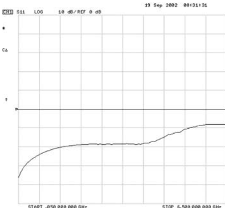
Figure # 23. Return loss tested to 6.5 GHz for the Reed Relay shown in Figure # 9. Horizontal full scale: 6.5 GHz. Vertical scale: 10 dB/div referenced from the 0 mark.
